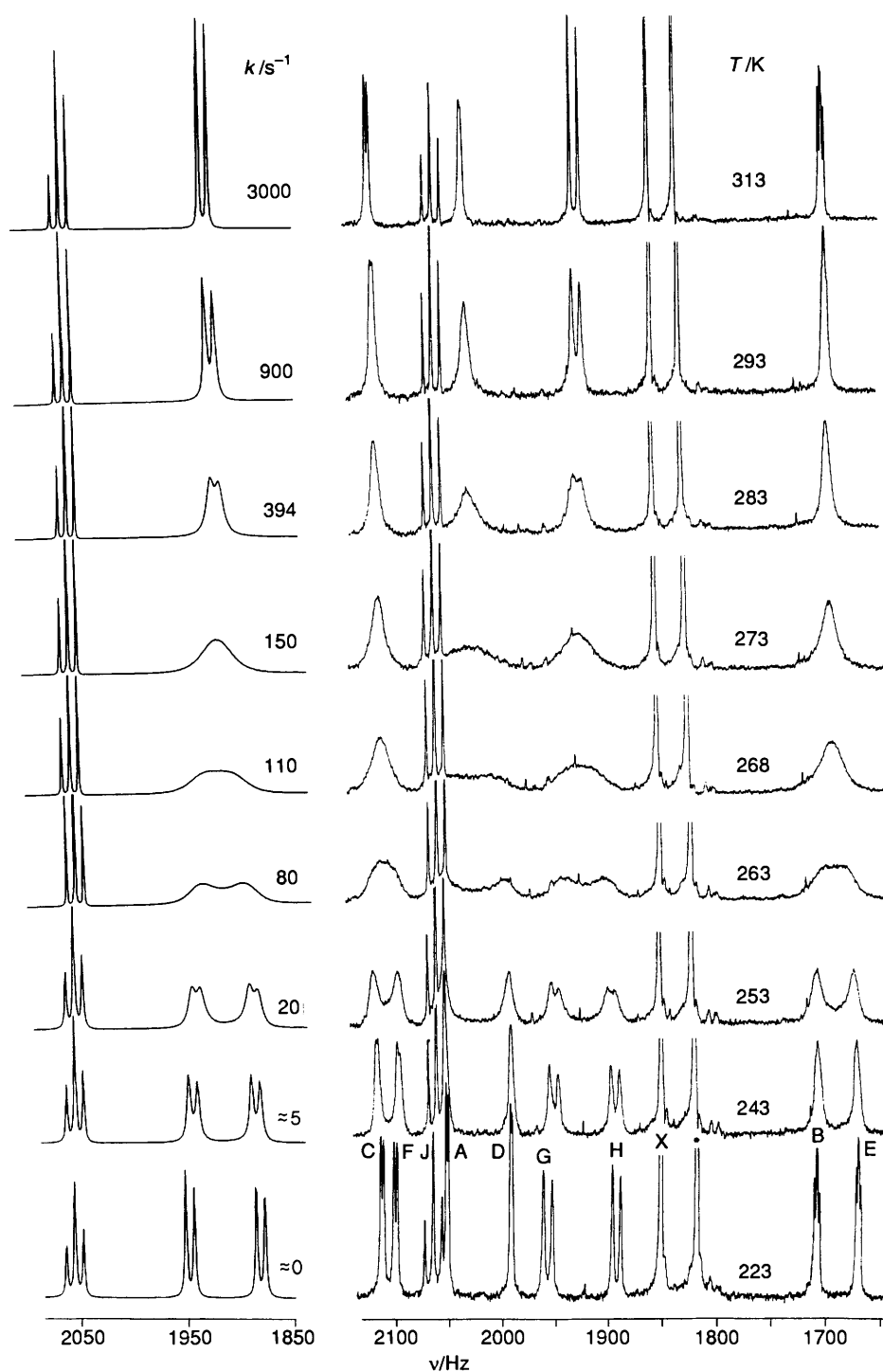
Fig. 5 Variable-temperature ^1\text{H} NMR spectra of [\text{ReCl}(\text{CO})_3(\text{bppy})] in \text{CDCl}_3 . See Table 3 for signal labelling. Signals marked X and \bullet are due to traces of \text{C}_6\text{D}_5\text{H} and \text{CHCl}_3 respectively. Computer-synthesised spectra of the pyridyl hydrogens are shown on the left
